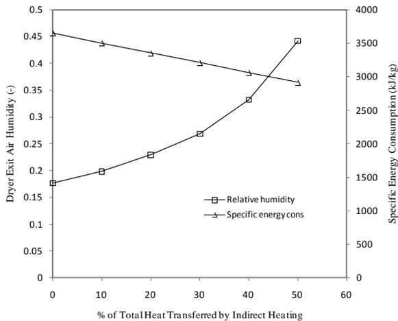
Fig. 8. Effect of indirect heating on exit humidity and specific energy consumption
