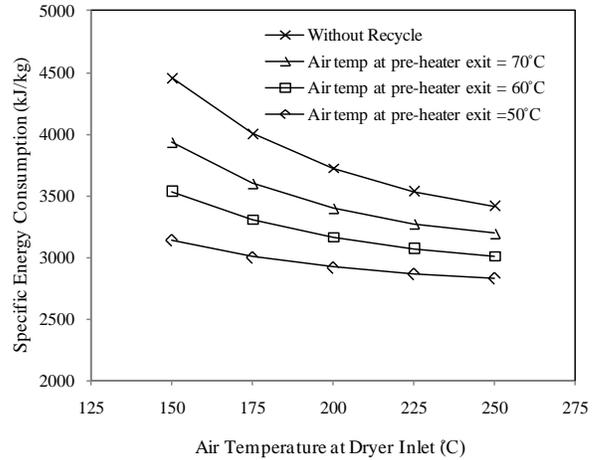
Fig. 4. Effect of pre-heating of fresh air on specific energy consumption
