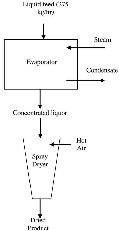
Fig. 9. Spray drying system used for study
