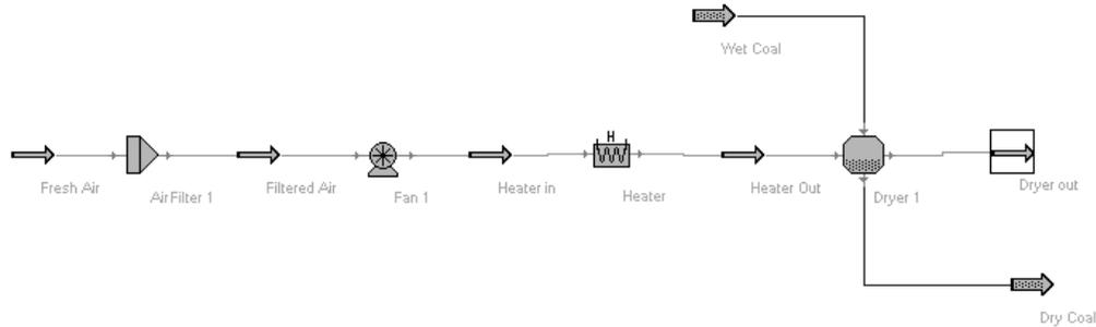
Fig. 1. Flow-sheet for a simple coal drying system
