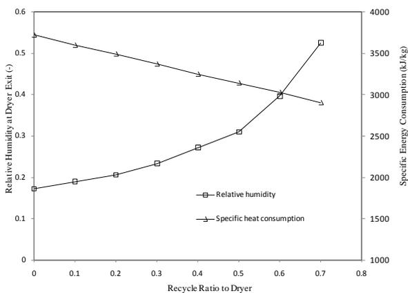
Fig. 6. Effect of recycle ratio on exhaust air humidity and specific energy consumption
