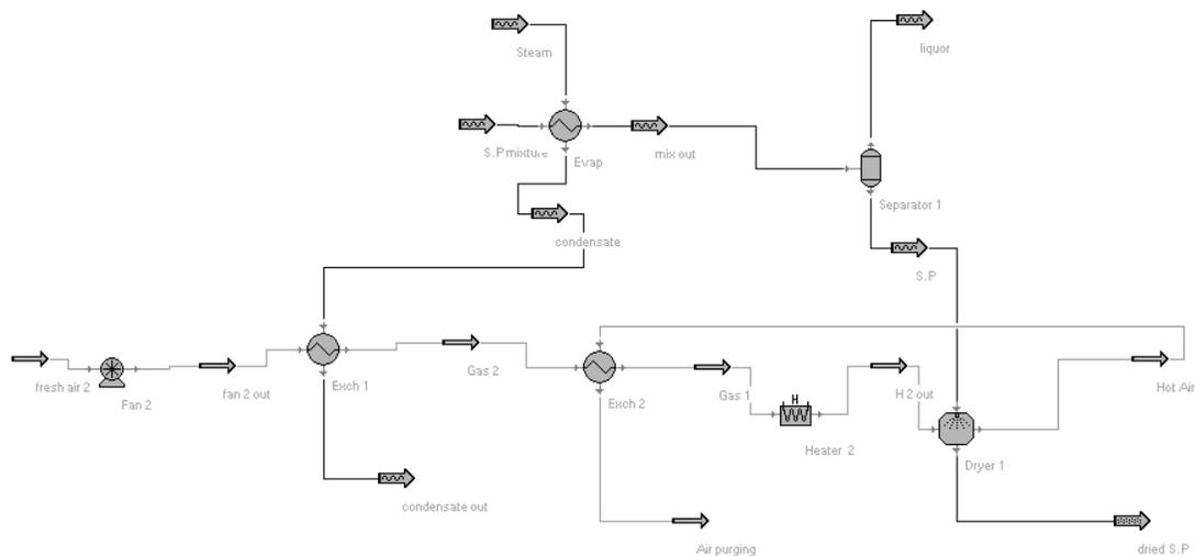
Fig. 11. Recovery of heat from condensate and dryer exhaust air
