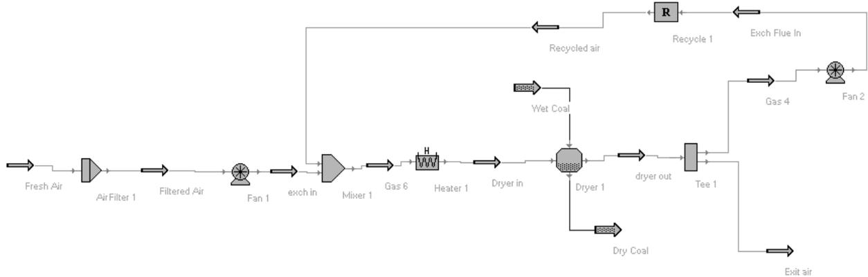
Fig. 5. Flowsheet for recycle of air to dryer
