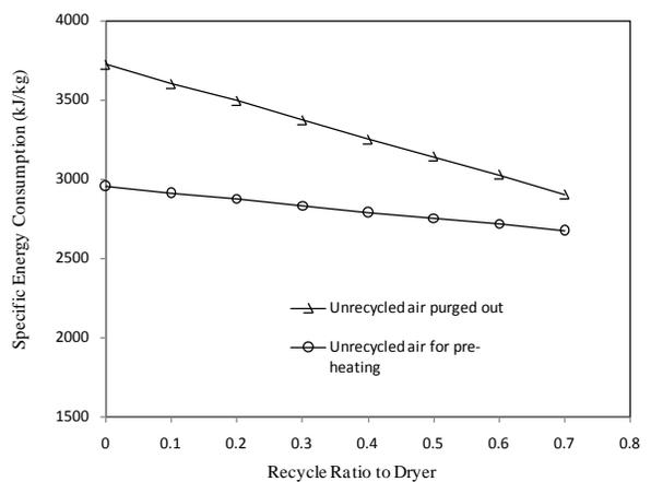
Fig. 7. Effect of recycle and pre-heating on specific energy consumption
