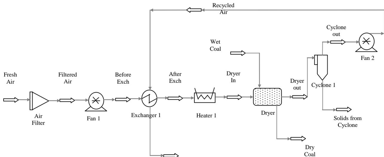
Fig. 3. Preheating of drying air using recycle air
