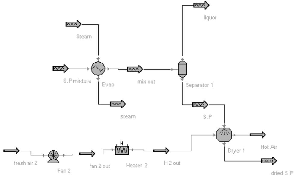
Fig. 10. Basic spray drying flowsheet used
