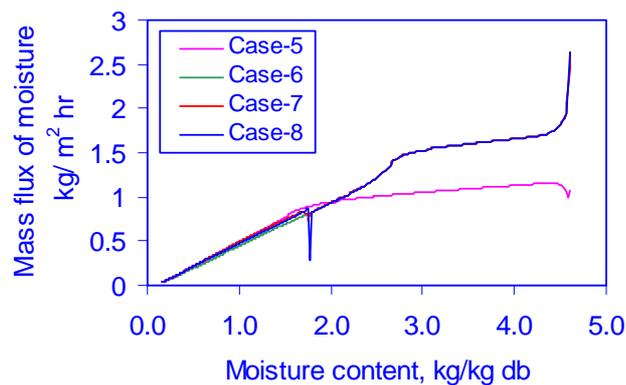
Effect of relative humidity of drying air: It is seen that dehumidified air using heat pump can improve drying rate at lower operating temperatures- a benefit for heat-sensitive materials. Results also show that heat pump is needed only in the initial drying period.
