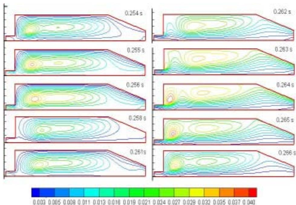
Figure 1 Gas flow pattern within drying chamber oscillate during a pulse combustion cycle (0.254-0.266 s, 81Hz)
