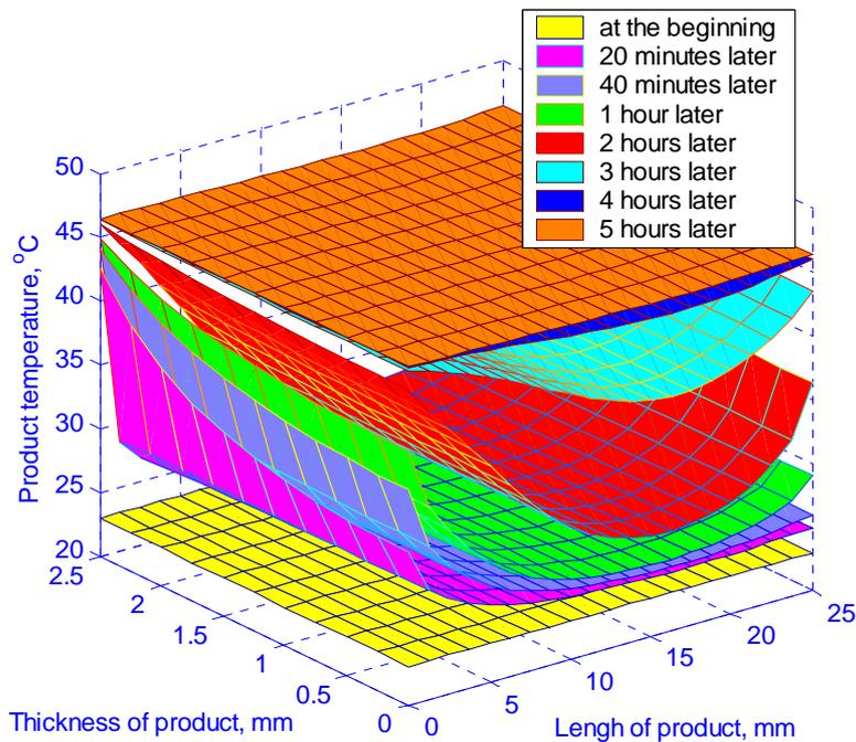
Predicted evolution of the temperature distribution inside a slab-like drying product using a 2D liquid diffusion model
