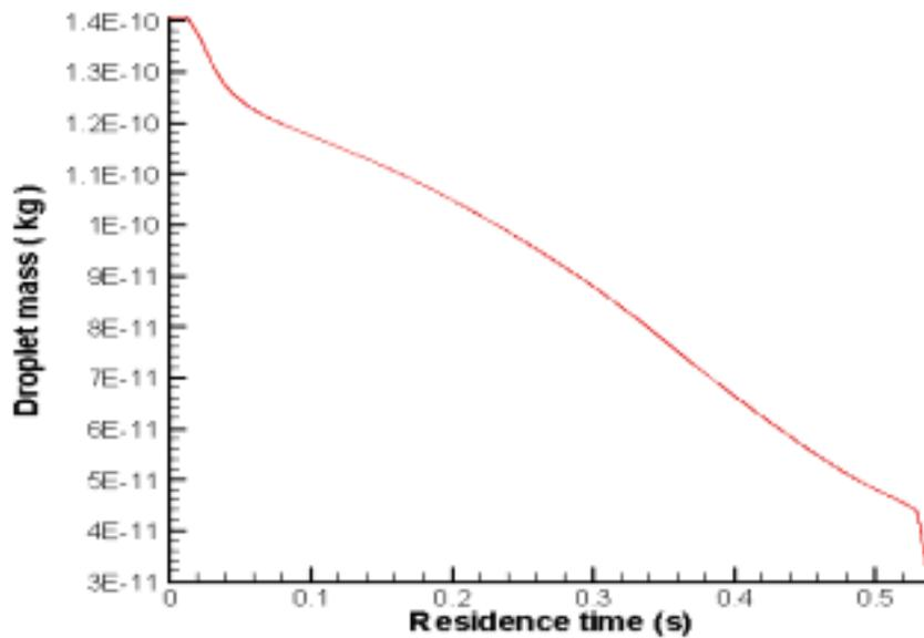
Figure 2 Droplet mass during the residence time after injected at  $t = 0.254\text{s}$  (droplet diameter  $D=63.1\times 10^{-6}\text{ m}$ , 10% mass fraction NaCl solution)
