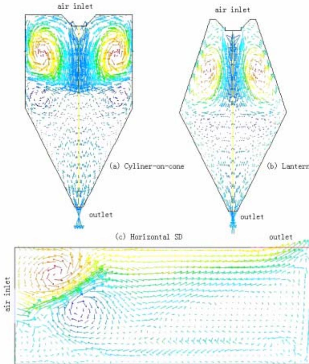
Figure 2-1 Air flow pattern in different geometries
