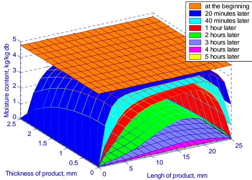
Predicted evolution of the moisture distribution inside a slab-like drying object using a 2D liquid diffusion model
