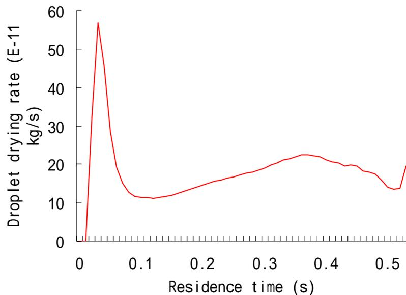
Figure 3. 13 Droplet drying rate during the residence time after injected at  $t = 0.254\text{ s}$  ( $D=63.1\times 10^{-6}\text{ m}$ , 10% mass fraction NaCl solution)
