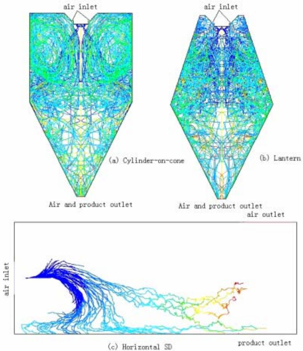
Figure 2-2 Particle trajectories in different geometries
