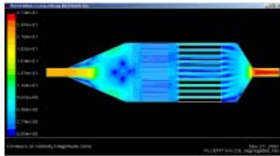
**Flow distribution inside the drying chamber fitted with multiple trays which are stacked with spacing between them for dehumidified hot air to pass between them.**
