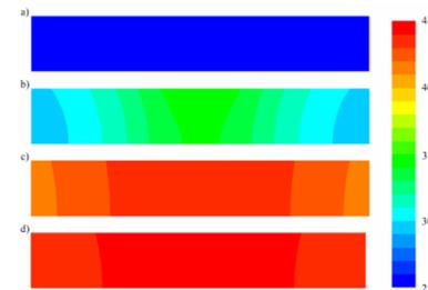
Figure 3. Temperature contour of impinging jet drying substrate
