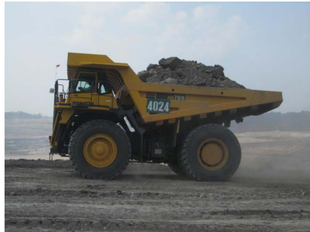
Truck which can carry up to 100 tons of coal
